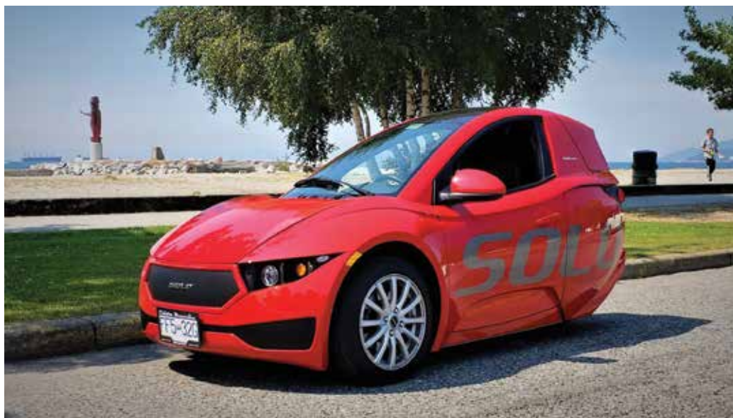
The Electra Meccanica Solo single-seat, three-wheel electric car is manufactured in Vancouver, British Columbia, Canada. In addition to its dealership in downtown Vancouver, its first US dealership is located in the Los Angeles suburb of Studio City. Powered by a lithium-ion battery, the car goes zero to 100 kph in eight seconds with a top speed of over 130 kph with a 160-km (100 mile) range. Retail price is CDN $19,888 (US $15,500). A two-seat roadster is in the works. Photo courtesy Electra Meccanica Vehicles Corp.
