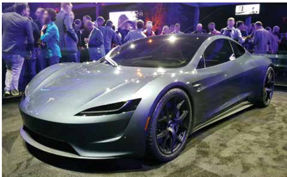
A prototype of the 2020 Tesla Roadster. The four-seater vehicle will accelerate 0-60 mph in 1.9 seconds. With its 200 kWh battery pack, the car has a range of 620 miles. Photo courtesy Tesla, Inc.
